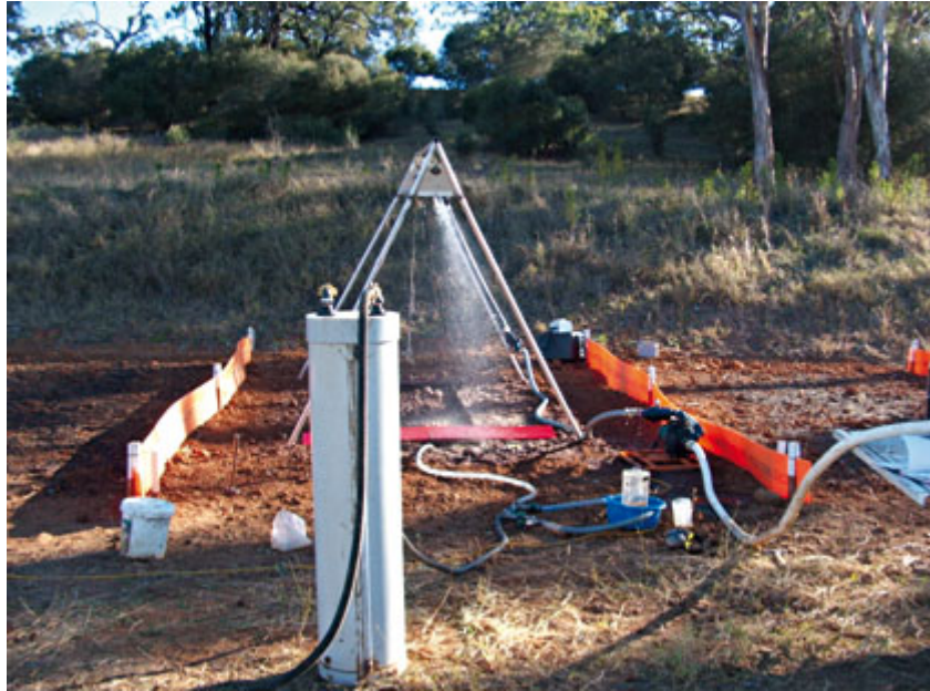
Figure 25. Illustration of the rainfall simulator used to deliver a 1 in 10 year rainfall event to runoff plots as part of the experiment.
